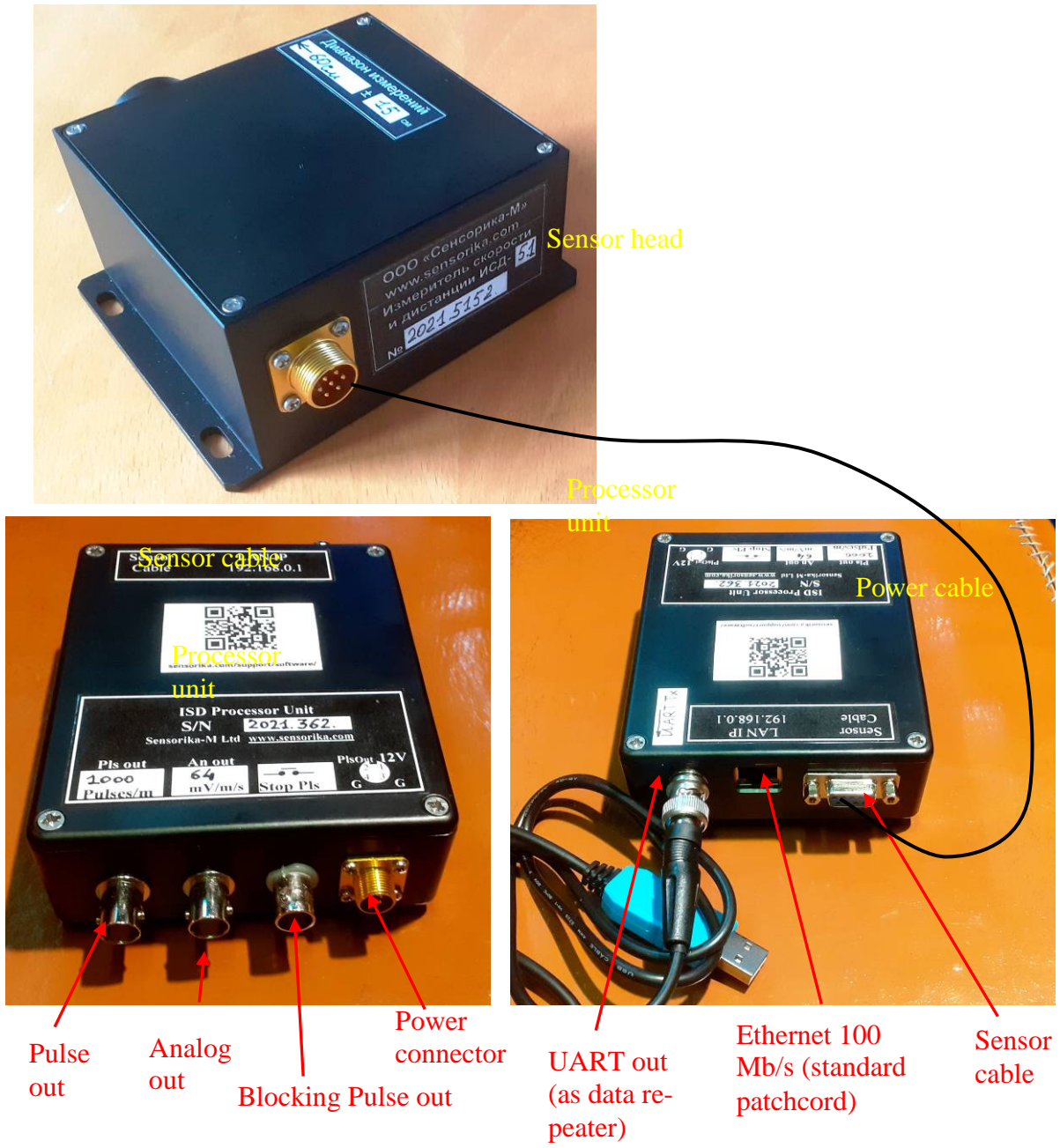
Fig. 1. Sensor parts and connectors.
