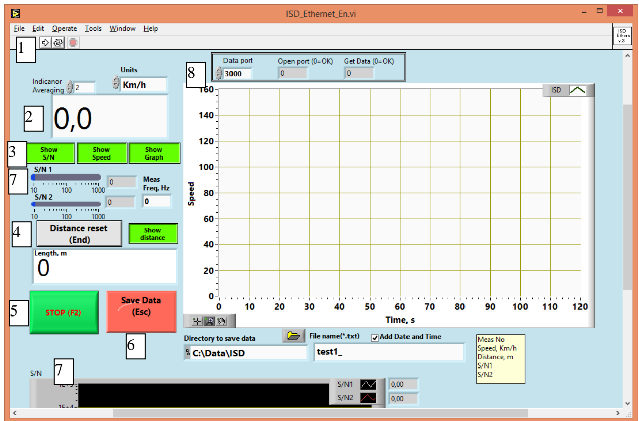
Fig.5. ISD_Ethernet_En.exe – Program to work with sensor data sent from controller to PC via Ethernet connection.
